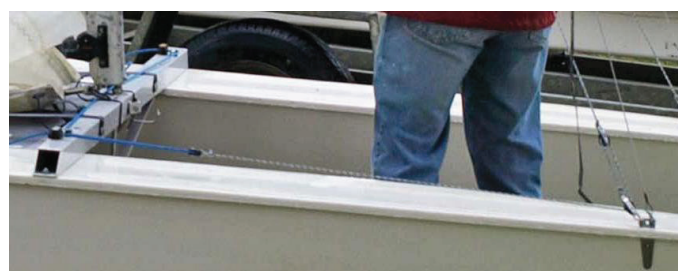
Externally mounted 2:1 plus 2:1 system
