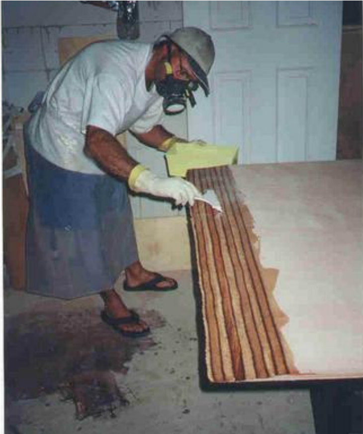
^ Apply Glue to all 4 ply tapers in one operation.
