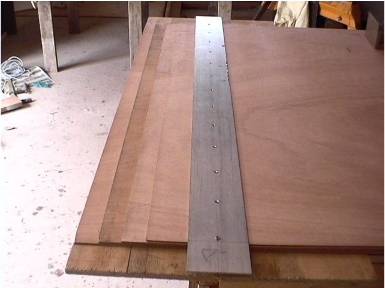
^ Stacking the plywood with the 40mm exposed.
