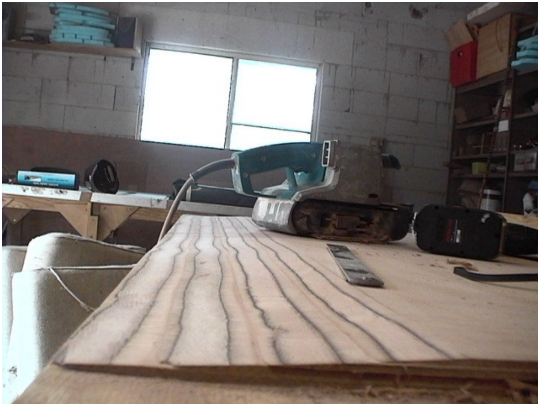
^ Taper finished - ready to glue to make scarf joint.
