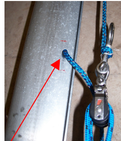
Hole for halyard rope to exit from mast track.
