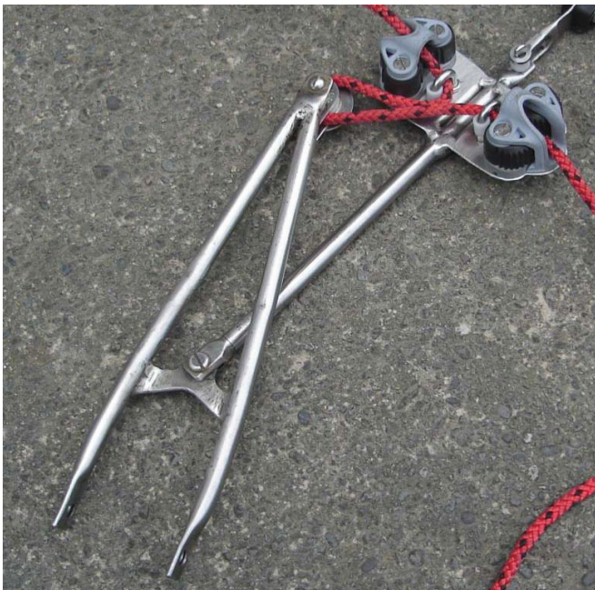
Modified spanner - control system on vang
