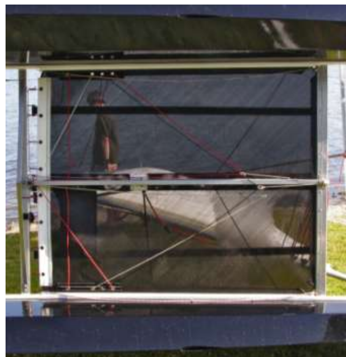
Example of endless systems for the downhaul (white), outhaul (black), vang (red to rear) and lower forestay (red forward) below the trampoline, with elastic take-up in the centrebeam.
