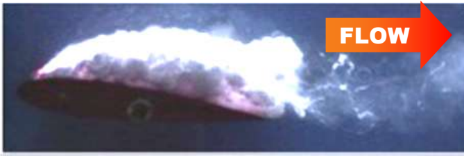
Example of cavitation (University of Minnesota)
