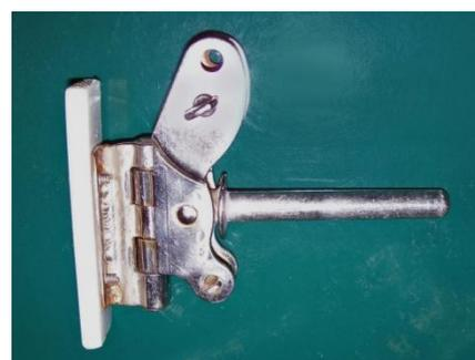
Welded plate and Nylon slide
