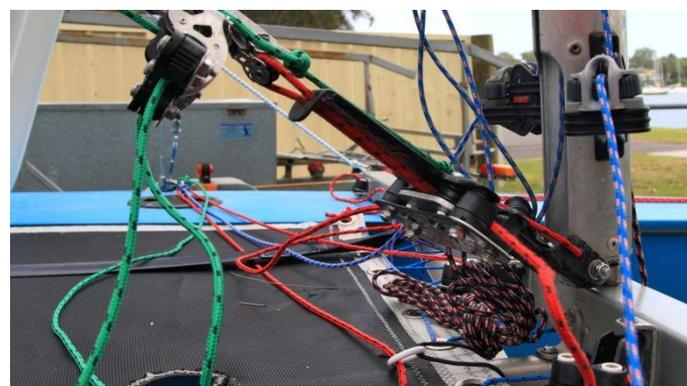
**Combination of tails tied to chainplates and an endless system**
