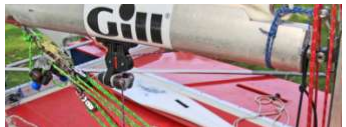
DOUBLE SWIVEL CLEAT WITH OUTHAUL AT THE REAR, AND LEECH CORD AT THE FRONT
