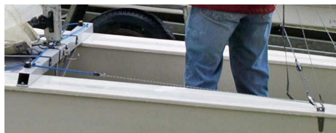
Externally mounted 2:1 plus 2:1 system
