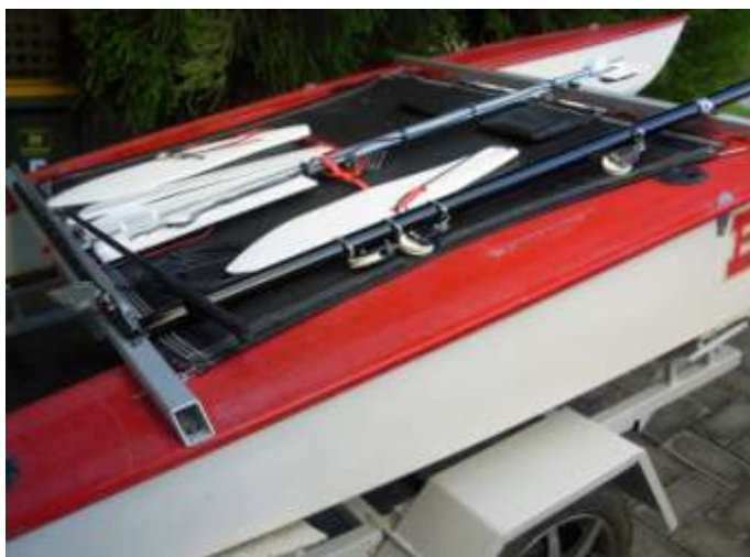
The trampoline arrangement showing tensioning wires
