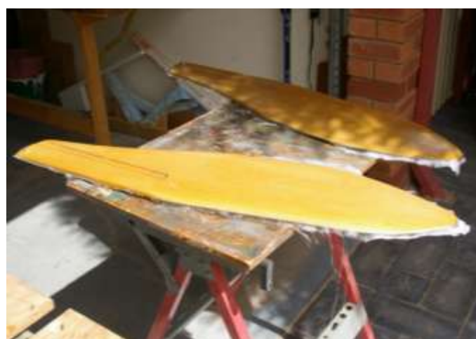
Jelutong rudders and centreboards after glassing
