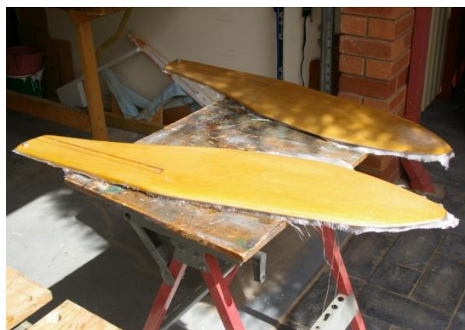
Jelutong rudders and centreboards after glassing
