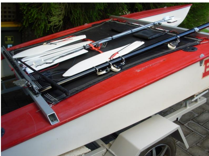
The trampoline arrangement showing tensioning wires
