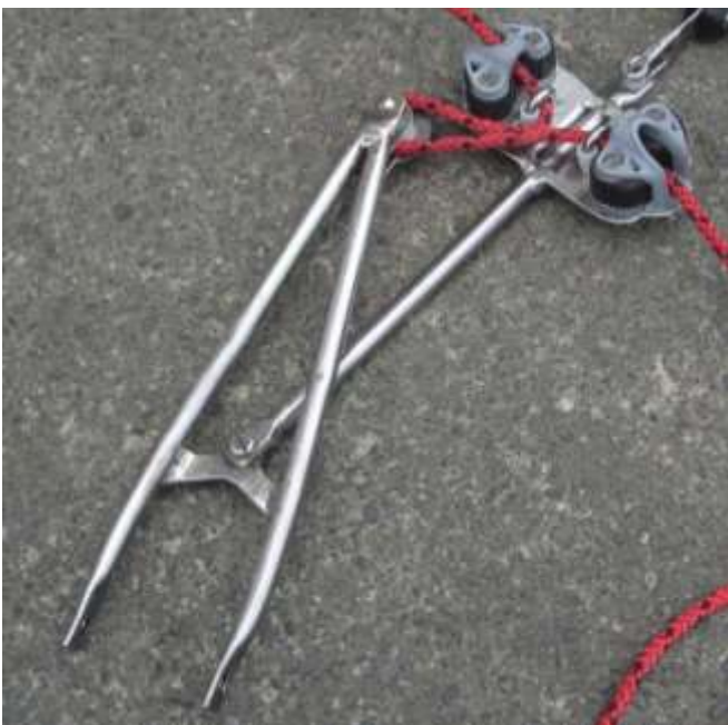
Modified spanner - control system on vang
