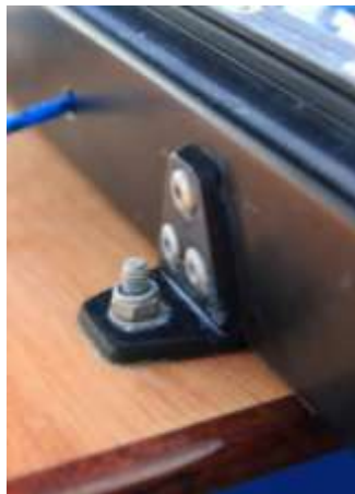
NZ style inner beam bolt
