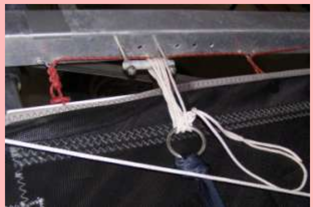
Jury rigged strap using a towing ring
