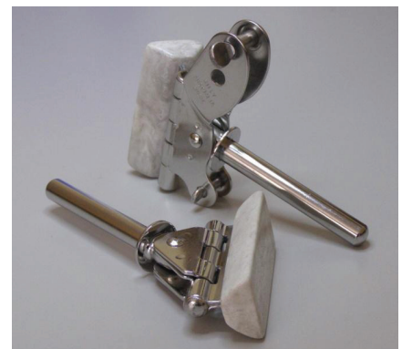
Goosenecks to suit either boom or sail attachment of downhaul (PT Shop)
