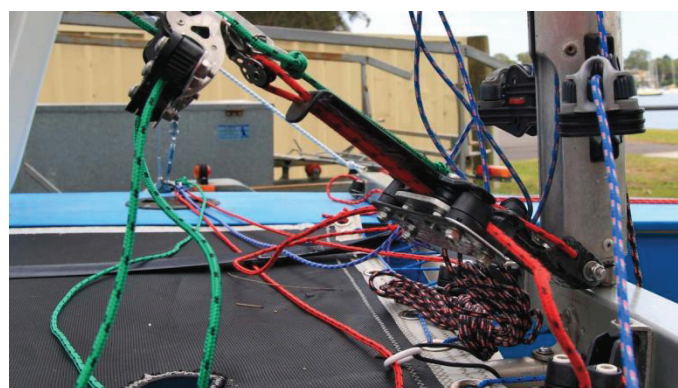
Combination of tails tied to chainplates and an endless system
