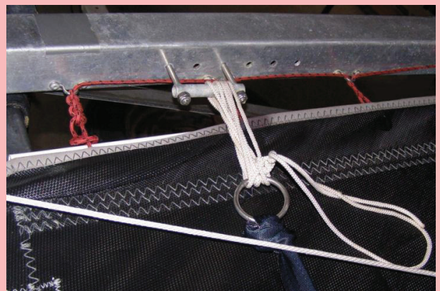
Jury rigged strap using a towing ring
