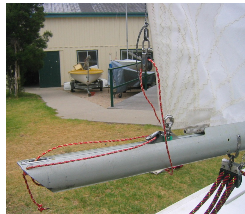
< Outhaul system shown in conjunction with leach-line system
