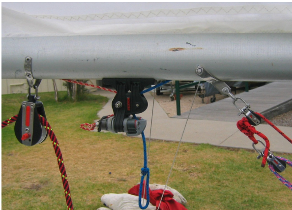
< Shows use of swivel cleats on boom and also rope exiting through slot in boom. This swivel has two cleats mounted back to back with one for the outhaul and one for the leach line.
