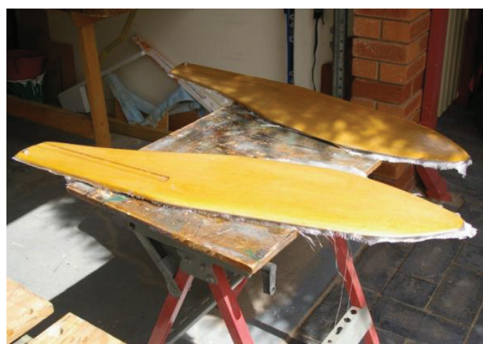
Jelutong rudders and centreboards after glassing
