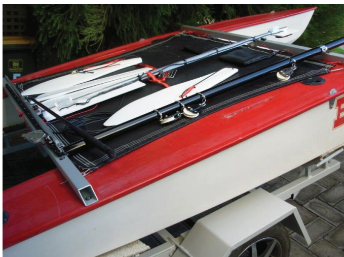
The trampoline arrangement showing tensioning wires
