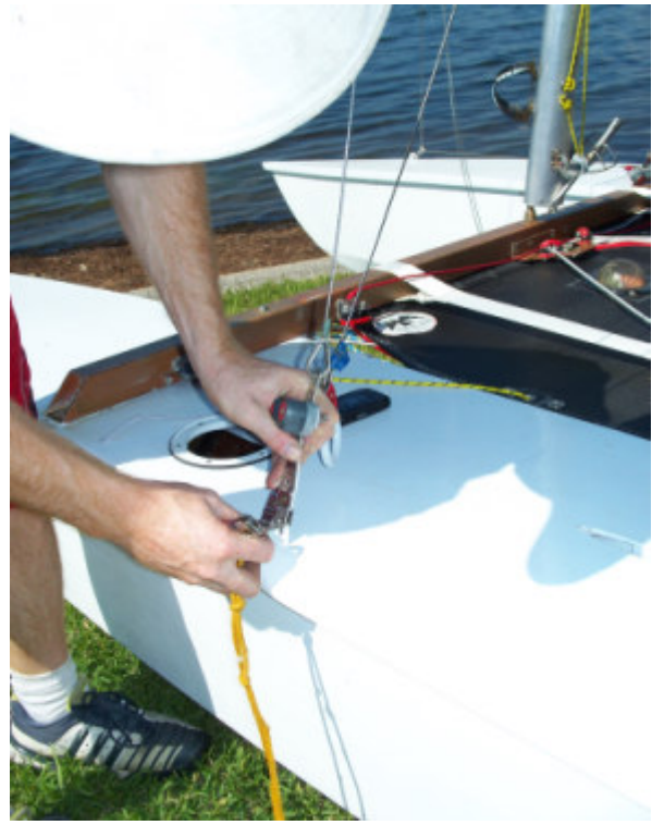
^ Attaching the final stay. If the boat has any amount of rig tension, use the method described above to help.
