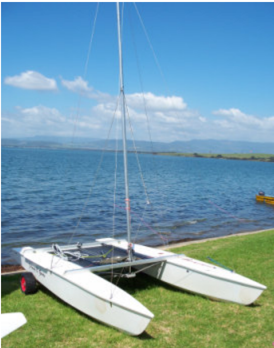
^ Here the boat has all the lowers attached, with just enough tension on the front lowers to keep the mast in position. The sailor is about to attach the other stays.
