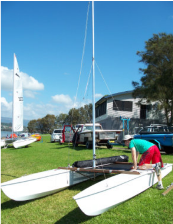
^ Here the boat has all the lowers attached, with just enough tension on the front lowers to keep the mast in position. The sailor is about to attach the other stays.
