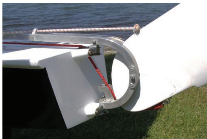
Tilting cleats outwards helps cleating from other hull
