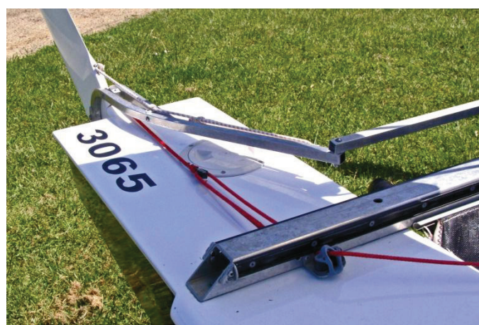
Tilting cleats outwards helps cleating from other hull
